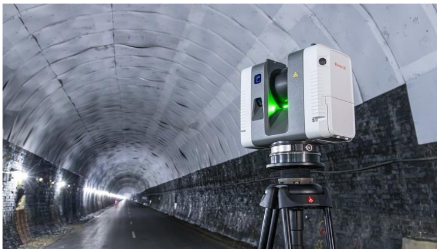
Figure 7: Laser pulse-based 3D scanning [9].
