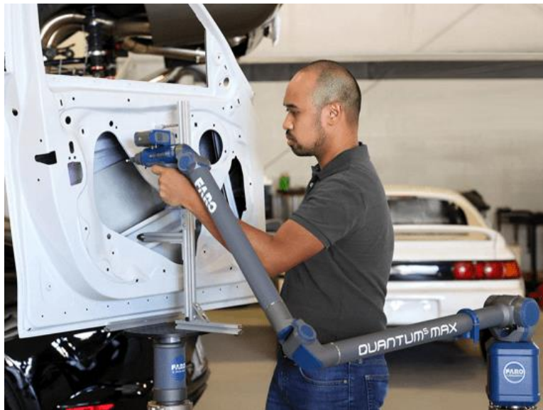
Figure 6: Contact 3D scanning [7].
