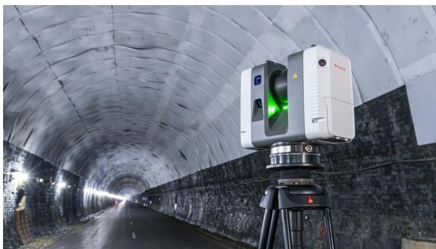
Figure 7: Laser pulse-based 3D scanning [9].
